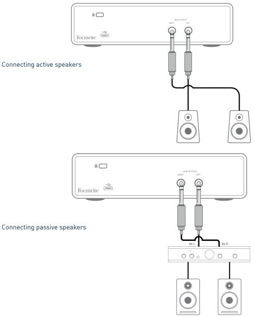
The line outputs are 3-pole (TRS) 1/4" (6.35 mm) jack sockets, and are electronically balanced. Typical consumer (Hi-Fi) amplifiers and small active monitors have unbalanced inputs, either on phono (RCA) sockets, or a 3.5 mm TRS jack plug to connect to a computer. In either case, use a suitable connecting cable with jack plugs at one end.
