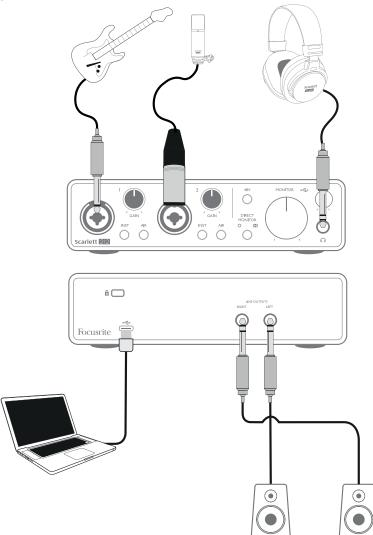
This setup shows the most typical configuration for recording with DAW software on your Mac or PC. You might record guitar through Input 1 and vocals through Input 2 into your DAW, while monitoring the playback from the DAW via headphones (or speakers).
